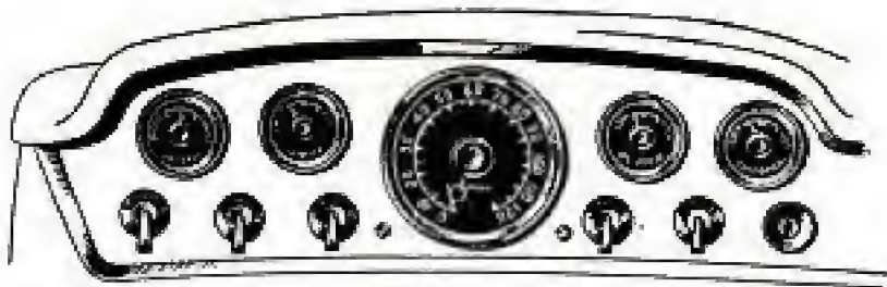
DESOTO has an instrument panel made up of perfect circles. Each instrument has a separate dial face for maximum clarity and visibility
